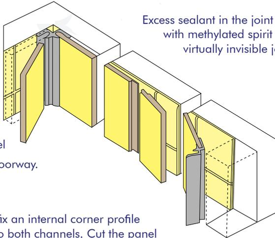
Excess sealant in the joint must be removed at once and then sprayed with methylated spirit and wiped with a damp cloth. This will ensure a virtually invisible joint.
