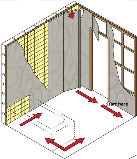
Fibo wall panels with Aqualock are fixed to battens/walls by nailing or screwing into the groove running along the length of the panel using No. 6 screws or 35mm gypsum board nails. Leave a distance of 200mm between each nail/screw. The lowest nail/screw must be fastened a maximum of 20mm from the bottom of the panel.
