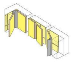
In areas of high humidity, Fibo panels must be fitted with a polymer waterproof sealant in every joint and to all exposed edges to ensure that they are totally waterproof. Apply the sealant when the panel is upright
