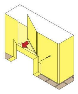
Cut the two panels left and right of the door so they have a centred space (full panel width) over the door frame. The last panel can be inserted tongue first on one side with the lip of the other edge removed to fit flush to the adjoining panel. Fix by gluing the back edge. Fit panels around the door frame with screws/nails which will be hidden by door moulding and coving.
