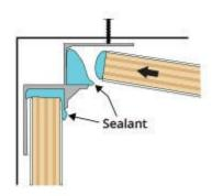
When setting up the first panel, fix an internal corner profile to the wall and apply sealant into both channels. Cut the panel to size and push the clean cut panel edge firmly into the profile.
