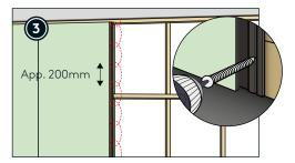
Affix with screws at a distance of approx. 200 mm. Recommended screws art. no. 810032.
