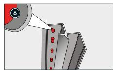
A small amount of sealant can be applied to act as a cushion between the profile and panel and reduce the risk of noise/rattling.
