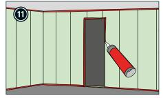
Apply fire-resistant sealant around the perimeter of the system to seal it.
