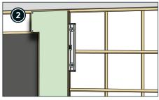
Start fitting above door. Ensure that the first panel is level.
