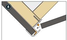
Apply sealant to the external corner profile to reduce noise and improve its grip.
