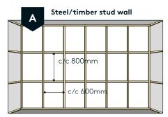
Timber or steel studs with recommended spacing as shown in the illustration.
