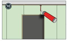
Apply fire-resistant sealant to the end joint above any doors.
