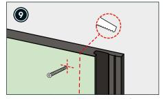
Cut to size and remove the click lock from the last panel.
