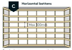
For the battens we recommend using formwork timber min. 21x98 mm or plywood 12x200 mm. Affix the Vito Fire Panel with two screws on each batten.
