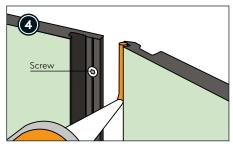
You can use Fibo Seal on the click lock to reduce the risk of cracking after drying. Not required.
