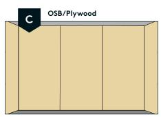
May be installed horizontally or vertically. Minimum recommended thickness is 15 mm OSB or 12 mm plywood. No need for noggings behind the sheets. Vito Fire Panel can be fixed directly onto the sheets.
