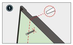
Remove the click lock on the left-hand side of the first panel. The red cross shows the location of the screw.
