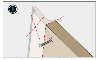
Clean cut first panel. Fasten to the back wall with screws or staples.
