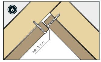
Fasten last panel against corner with screws or staples. The screw/staple will be hidden with putty or acrylic sealant.
