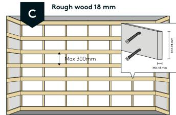
Horizontal battens (e.g., rough wood) with a maximum spacing of 300mm between battens.
