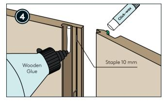
Use wooden glue and Click-wax as shown. Use a gentle rocking movement to prevent damage when connecting the panels. Remove any glue residues from the surface with a damp cloth.
