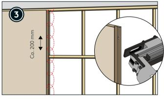
Ideal screw/staple distance is approx 20 cm. It is recommended to use staples in the click lock to prevent cracking of the wood fibers.
