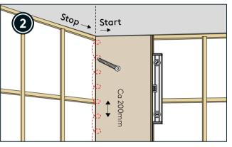
Make sure you fit the first panel plum. Fasten with screws or staples. Between floor/wall and floor/ceiling leave a 5 mm expansion gap.
