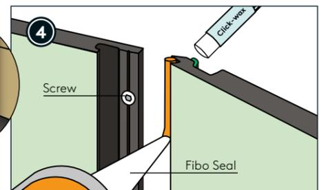
Use Fibo Seal on the click-lock to reduce the risk of cracking after drying. Use Fibo Click-wax behind the click (ref. image no. 12)
