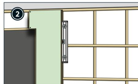
Start fitting above door. Ensure that the first panel is level.
