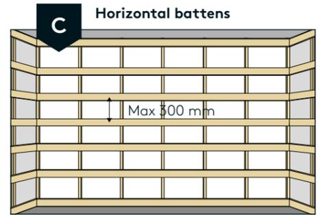
For the battens we recommend using formwork timber min. 21 x 98 mm or plywood 12 x 200 mm. Affix the Vito Fire Panel with two screws on each batten.
