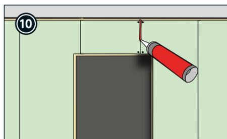
Apply fire-resistant sealant according to EN 1366-Part 4 in the panel joint above the door.
