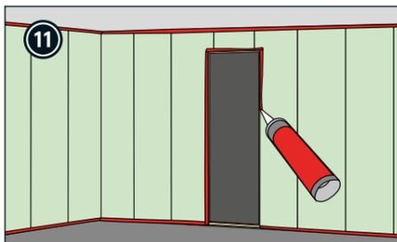
All transitions/gaps needs to be sealed with fire-resistant sealant according to EN 1366-Part 4.
