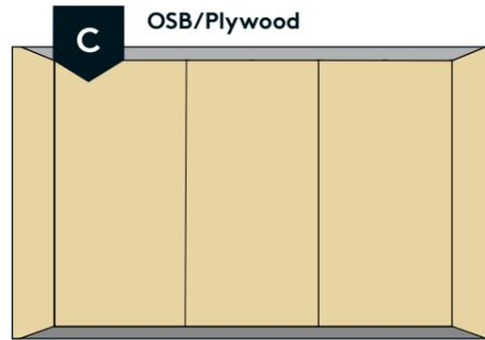
May be installed horizontally or vertically. Minimum recommended thickness is 15 mm OSB or 12 mm plywood. No need for noggings behind the sheets. Vito Fire Panel can be fixed directly onto the sheets.
