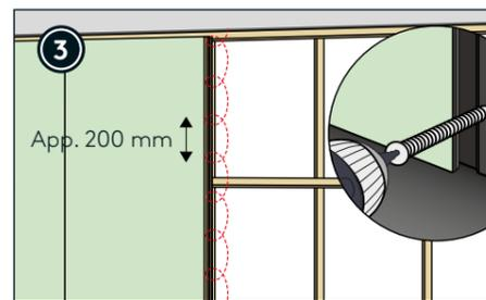
Affix with screws at a distance of approx. 200 mm. Recommended screws art. no. 810032.
