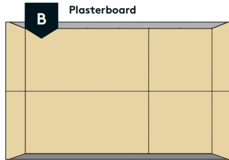
We recommend fitting plasterboards horizontally due to the seams. Min. 12.5 mm thickness. Add noggings at intervals of cc 800 behind the plasterboard, alternatively use two layers of plasterboard. Affix the boards to the studs behind.
