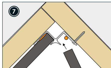
Apply sealant to the internal corner profile to reduce noise and improve its grip.
