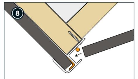
Apply sealant to the external corner profile to reduce noise and improve its grip.
