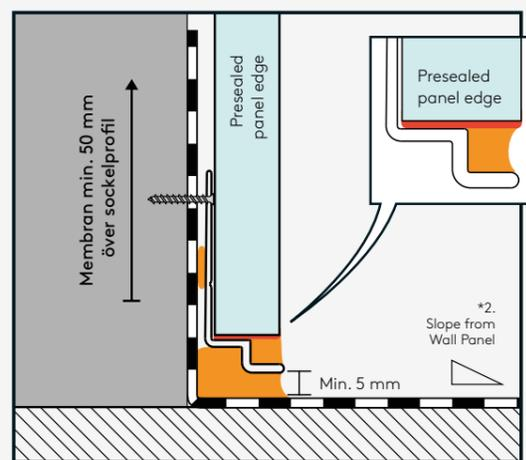
When installing the base profile, you can choose the height at which to mount the base profile depending on whether the room has a floor drain or not.
