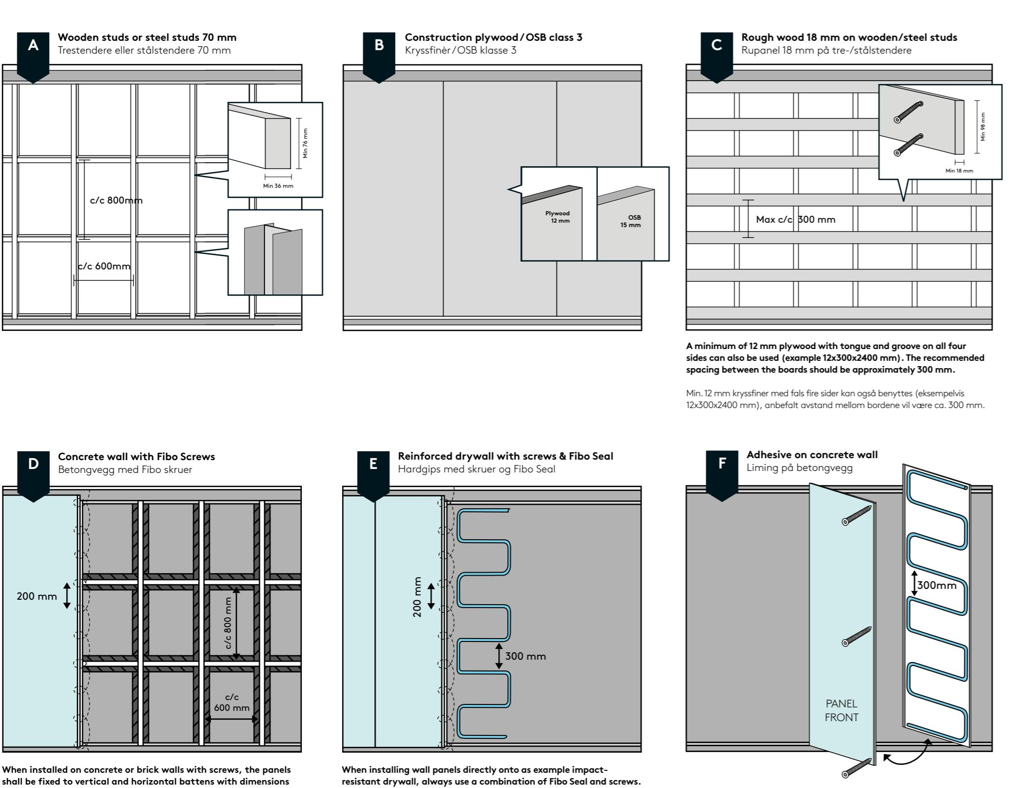
When installed on concrete or brick walls with screws, the panels shall be fixed to vertical and horizontal battens with dimensions min. 25 mm x 48 mm. The battens shall be installed c/c 0.8 m with the wide side flat, with a capillary obstructing layer between the inner battens and the concrete wall.
