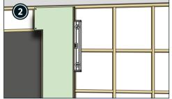
Start the installation above door. Ensure that the first panel is level.
