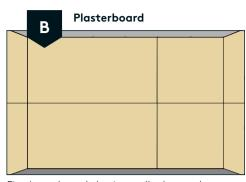
Fit plasterboards horizontally due to the seams. Min. 12.5 mm thickness. Add noggings at cc 800mm, or use two layers of plasterboard. Screw the panels through plasterboards and into the studs behind.
