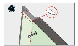
Remove the click lock on the left-hand side of the first panel. The black cross shows the location of the screw.
