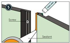
Use sealant on the click-lock to reduce the risk of cracking after drying. Use Fibo Click-wax behind the click (ref. image no. 12)
