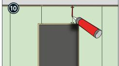
Apply fire-resistant sealant according to EN 1366-Part 4 in the panel joint above
