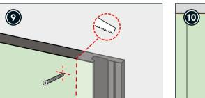
Cut to size and remove the click lock from the last panel.
