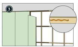
For wet rooms sealant is required behind the panels. Apply onto horisontal strips as shown.
