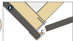
Apply sealant to the external corner profile to reduce noise and improve its grip. Screw the profile to the back wall as shown above.
