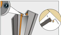
Apply sealant to the internal corner profile as shown above, to reduce noise and improve its grip. Slide into place and fasten corner profile with screw into back wall.
