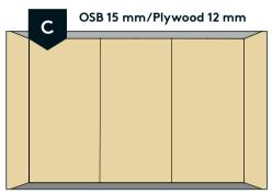
May be installed horizontally or vertically. No need for noggings behind the sheets. Screw the panels directly onto the sheets.
