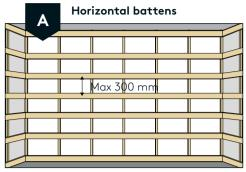
For battens use min.  $21 \times 98$  mm rough wood or  $12 \times 200$  mm plywood. Fasten the panel with two screws into each batten.
